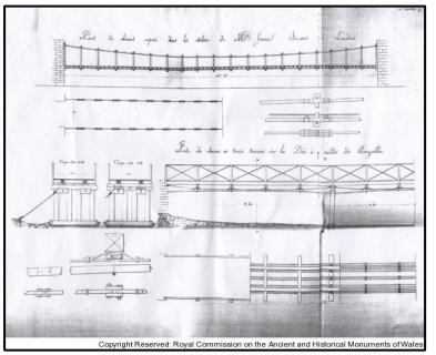
Pickering's bridge was constructed of wooden decking supported by wrought iron chains from below. This was then capped with earth and stone to give a form of roadway. Six oak pillars also supported the bridge over river bed, substantial enough to withstand heavy floodwaters.
